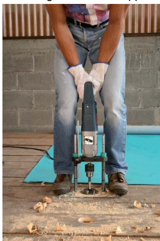
Ø 65 mm self feed wood bit
